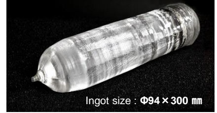
Fast-LGSO (Ce-doped \text{Lu}_{2-x}\text{Gd}_x\text{SiO}_5 )
